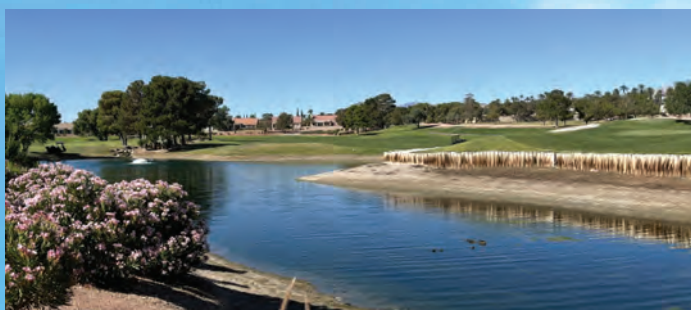
Renovations at Lake 10 at Palm Valley have been completed (the lake was drained, reshaped and the liner was replaced).
